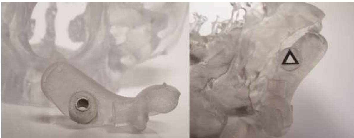
Figure 66 – Benchmark (left) and one of the developed guide (right) example, Benchmark guide is a SLA Clear jacket with a stainless steel insert and the developed guide is 2.95mm triangle cobalt chrome AM insert in a SLA Clear jacket.
