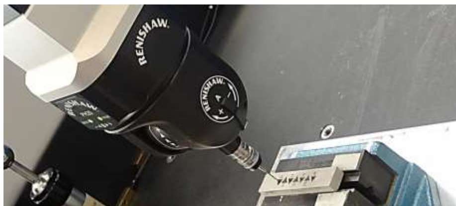
Figure 57 – Renishaw Plc. CMM was used to calculate the angulation and build error of each test bar. The CMM gathered three readings at -1mm, three readings at -4mm and three readings at -7mm.
