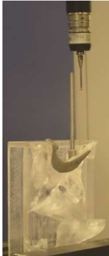
Figure 69 – Renishaw Plc. CMM was used to calculate the angulation error of each of the benchmark and developed surgical guides using the datum block as constant stationary object clamped into the vice. The CMM gathered six readings at -5.5mm, six readings at -10mm and six readings at -14mm.
