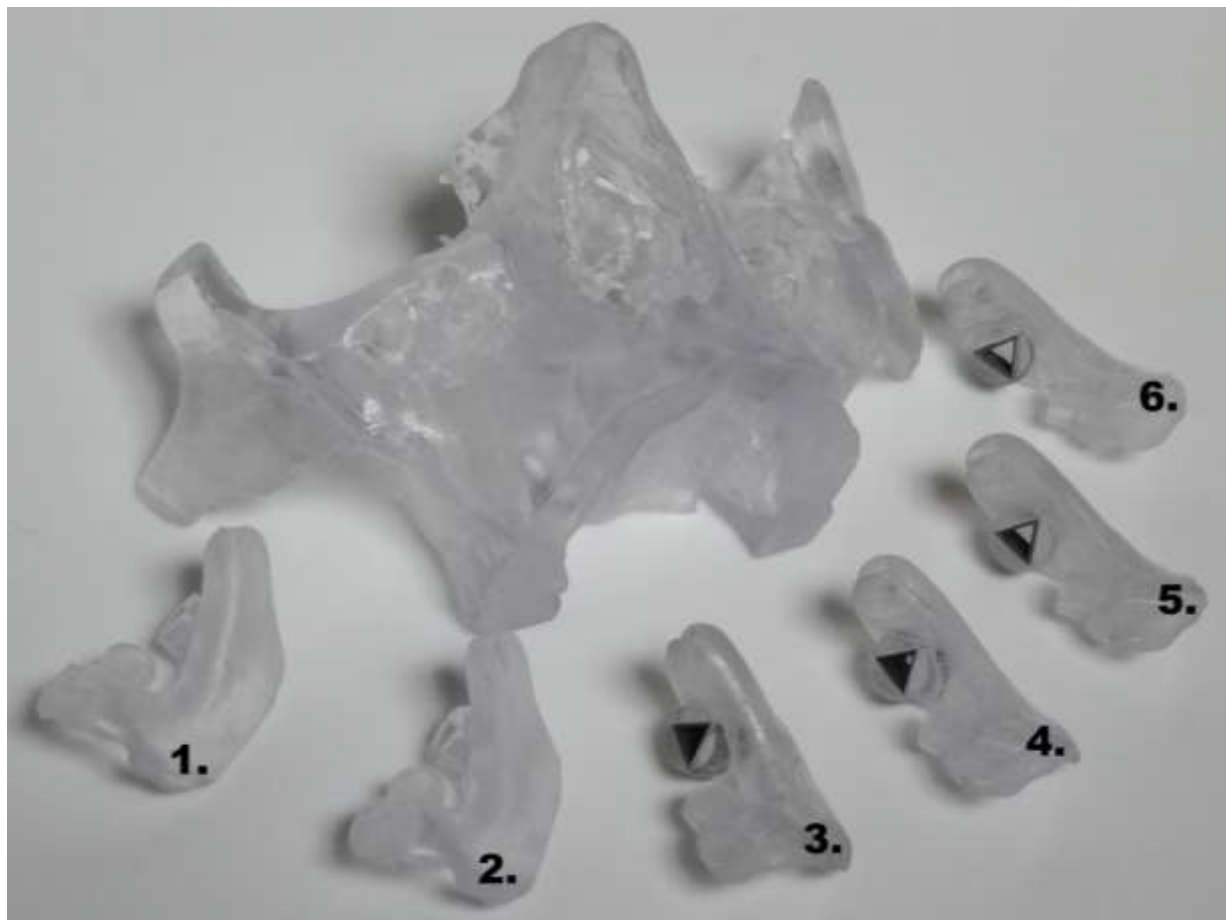
Figure 67 – The six developed nasal surgical guides with different iterations and tolerances on the triangle geometry.
