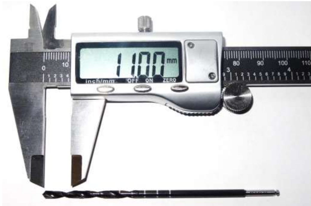
Figure 53 – The total length of the double start drill to complete a 360° pitch is 11mm, the measurement should influence the drill cylinder length and act as the minimum measurement in order to avoid inaccuracy due to the sway of the drill if the drill cylinder is designed less than 11mm.
