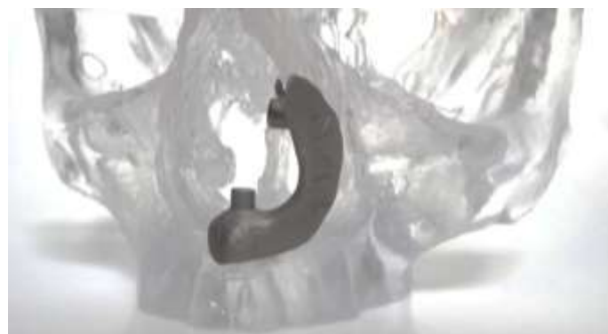
Figure 51 – AM cobalt chrome surgical guide which was trialed on the bone, but was not used on the benchmark guide patient. The guide was deemed too rigid around the nasal bone.
