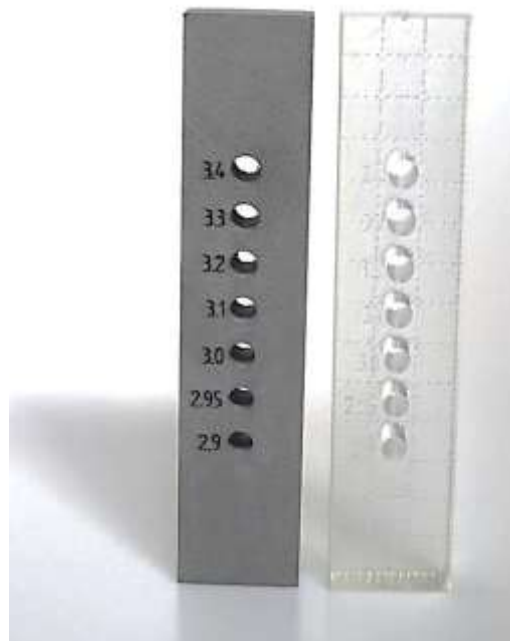
Figure 54 – Tolerance test bars fabricated using AM Cobalt Chrome and Visijet Clear. The tolerances on the circular diameter are 0, 0.05, 0.1, 0.2, 0.3, 0.4 and 0.5mm in each. For best results of the circles geometries the test bars were built up facing.
